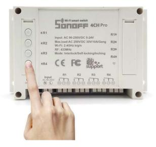
2. Press and hold one of the 4 switch buttons for 7 seconds until the wifi LED fast blinks 3 times and repeats.
