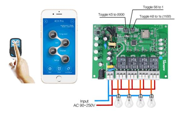
3. In interlock mode, you can turn on 1 device every time, and turn off other devices at the same time. For example, if you have turned on CH2, then when you turn on CH3, CH2 will be auto-turned off at the same time.
